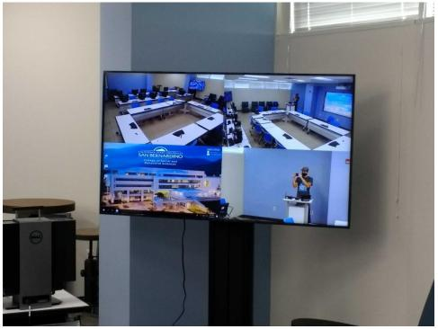
Enhanced presenter helper screen can be moved to several optimal locations in the room or allow it to be used for the remote presenter camera view. Additionally, camera and presenter views can be mixed and matched for a really highend production impression.
