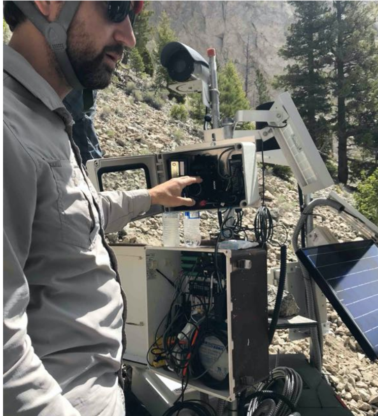
Figure 3. Joel Smith of the USGS describes Chalk Cliff monitoring instrumentation that consists of solar panel for power (right), long distance video camera (top), and controls in other boxes. Camera is monitoring station shown in Figure 4A and 4B.
