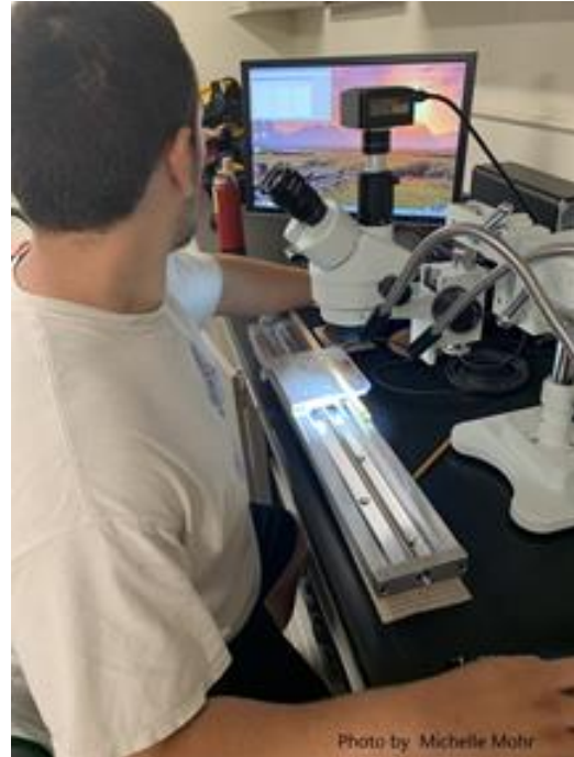
Figure 7. Student researcher Gabriel Angulo recording measurements of a sample using Velmex Tree-Ring Measuring System.
