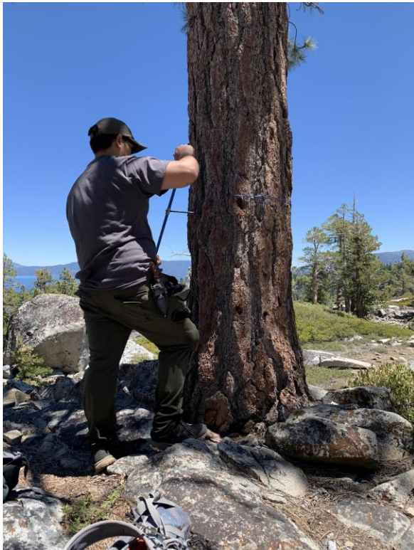
Figure 2. Student research Gabriel Angulo using increment borer to obtain core.
