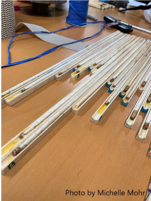
Figure 5. Samples were mounted onto wooden structures, which were custom made by CSUDH students in the Tree Ring Lab.
