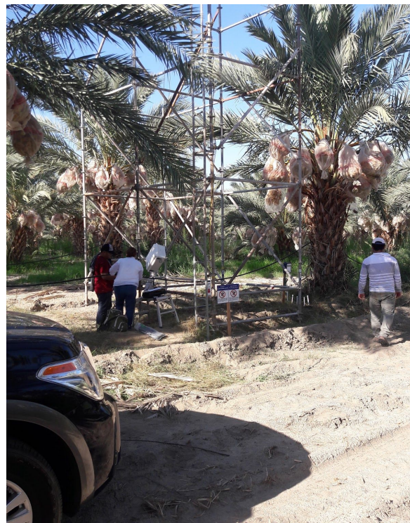
In this photo we are at a Date Palm site we are setting up soil moisture sensors, water mark box, and a weather/solar panel station up above the scaffold for data collection.
