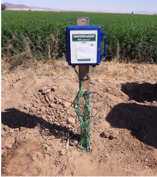
In the photo above is a watermark box we set up to connect the soil moisture sensors of different depths to gather data in the alfalfa fields.
