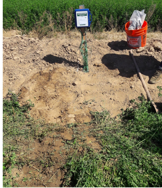
In the photo above is a pulled back view, the soil moisture sensors were dug underneath the soil in order to not get trimmed by the truck that harvests the alfalfa.
