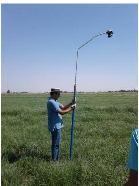
In this photo, I am taking inferred photos in a field of Klein grass. The photos form this field would go through a program that will analyze moisture content.
