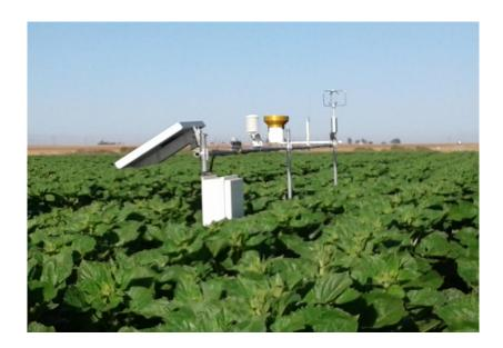
This is an example of our E.T weather stations that we would put in fields throughout in the Imperial Valley. These weather stations contain sensors that measure temperature, wind speed, dew point, rainfall, etc.
