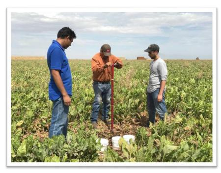
In this photo, our research lab assistant, Daniel Buenrostro, student from UC Riverside, Diego Jones and myself are using a soil auger to collecting soil samples from a sugar beet field in Westmorland, CA. This will allow us to test nitrogen levels and nutrients in the soil.
