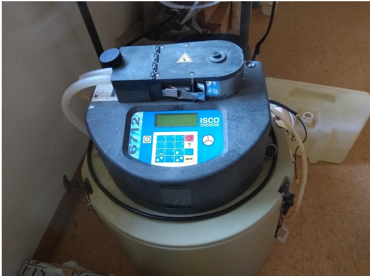
Image 3. This is an ISCO model 6712 water sampling device used during the tracer experiments. This device is also used to monitor flows, pH, and temperature of various creeks on site.
