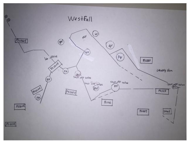
Figure 2 is a handmade sketch for the Westfall station located in the Madera County of the Sierra National Forest. The lines showing on the sketch are the water lines, the circle points are valves such as Butterfly Valve (BV) also the Well box (W). We also have the building numbers two tanks in the upper left corner and finally the Fire Hydrants (FH). Over all this is what a water system will look like.
