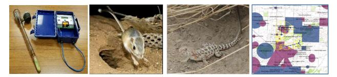
The picture above is a moisture sensor and a monitor. The sensor is equipped with a pressure gauge which reads the level of water suction on the sensor.
