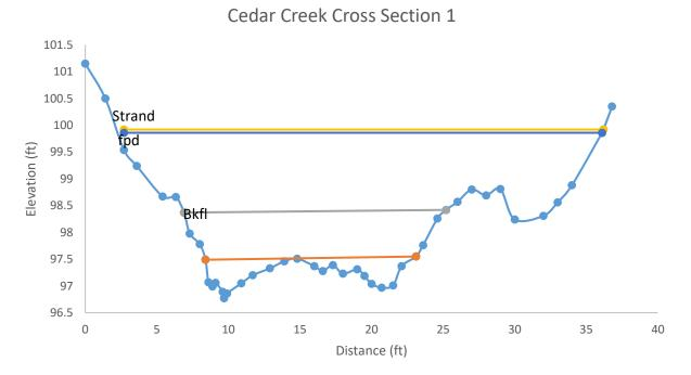
**Figure 2.** Cross section 1 taken at Cedar Creek showing the strandline, flood prone depth, bankful depth, and water surface elevation.
