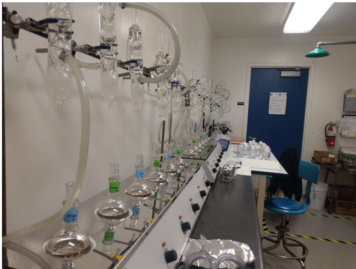
Soxhlet process set-up for extraction of compounds from microplastics or granular activated carbon.
