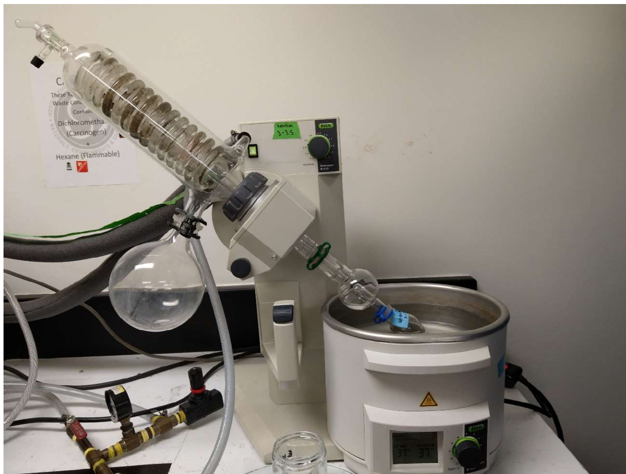
RotoVapor set-up for concentrating the final solutions for Gas Chromatography/Mass Spectrometry (GCM) analysis.
