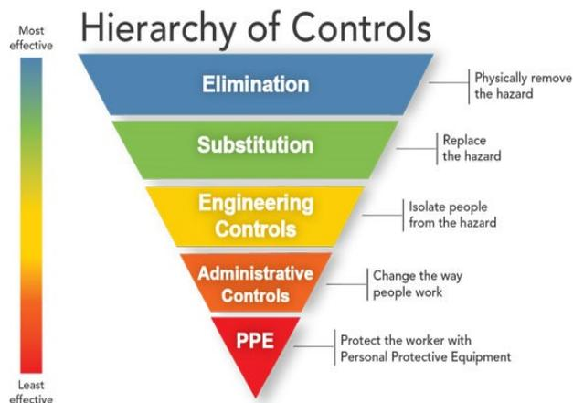
As shown in *Figure 2*, the Hierarchy of Controls is a methodology that helps us to understand the relationship between different control methods and their effectiveness at addressing a hazard. Controls at the top of the hierarchy are more effective than controls on the bottom. As it pertains to COVID-19 infection control procedures, we aim to apply this same methodology to understand what methods will be most effective in preventing the spread of COVID-19.
