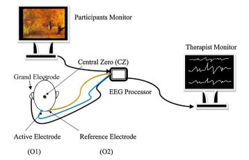
Fig. 1. Schematic illustration of the neurofeedback system. Electrode placement in the 10-20 electrode system on O1 & O2 which are left & right Occipitals of the scalp. Subjects play games without using hands and therapist control these games based on subjects' mental waves.
