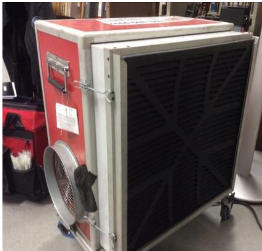
Air scrubbers were placed around the basement and 1F of the older portion of the library with HEPA filters and 1" pleated filters installed
