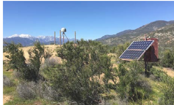
PBO site P612 at the CSUSB Land Lab. This site is part of a large network of Global Positioning System (GPS) instruments comprising the Plate Boundary Observatory (PBO) component of the EarthScope which precisely measures Earth deformation resulting from the constant motion of the Pacific and North American tectonic plates in the western United States. See: http://www.earthscope.org
