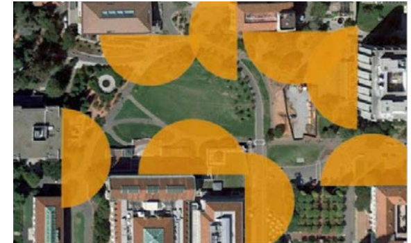
Example of 24-camera coverage map of public area producing 8,000,000 pixels of video information (left), as compared to a coverage map with 8 panoramic cameras supplying 96,000,000 pixels of video information (right).
