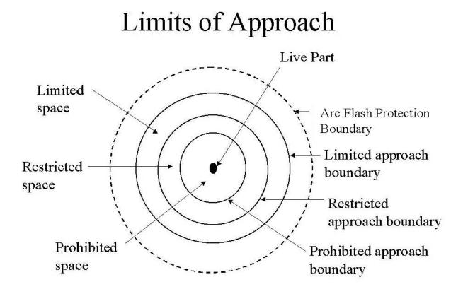
Note: The Limited, Restricted, and Prohibited Approach Boundaries are based on voltage. The Arc Flash Protection Boundary is based on the available incident energy equal to 1.2 cal/cm<sup>2</sup> (the onset of a second degree burn). The Arc Flash Protection Boundary may be less than or greater than the Limited Approach Boundary.
